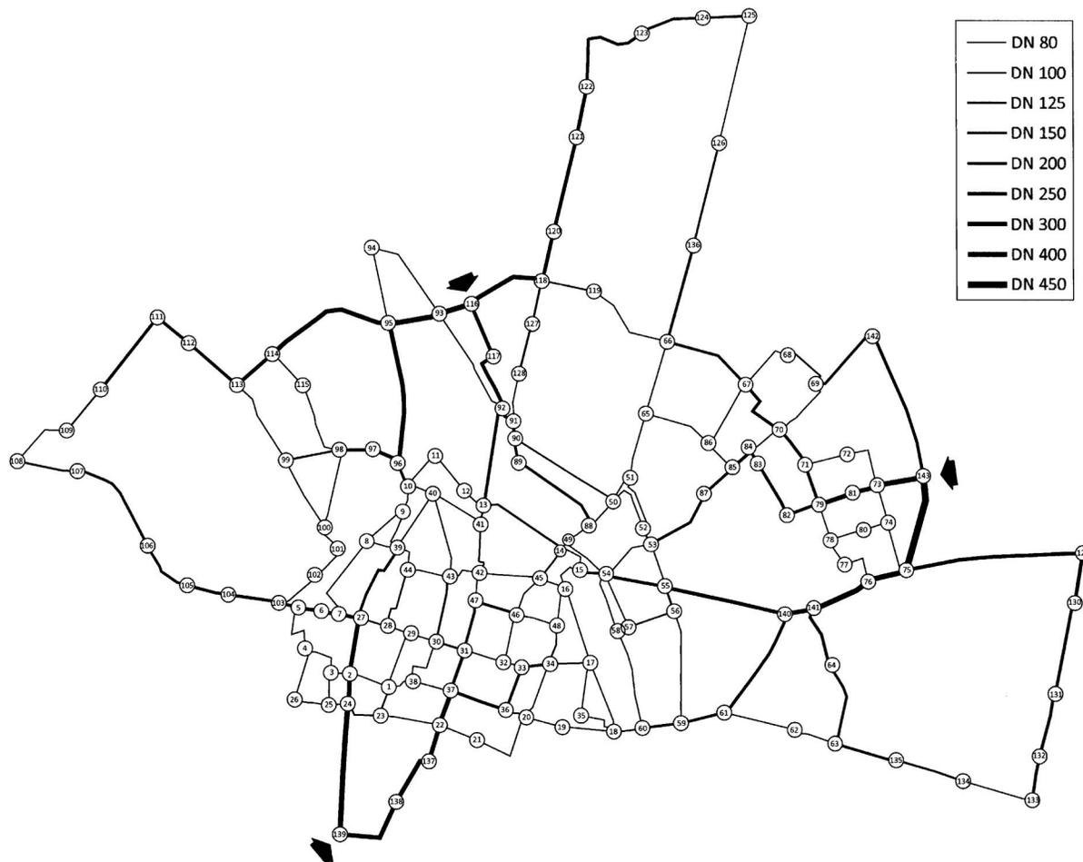
**Fig. 1.** Scheme of Pavia water distribution network (solution A)
